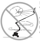
Do not raise the boom when wind speeds may exceed 12.5 m/s. If wind speeds exceed 12.5 m/s when the boom is raised, lower the boom and do not continue to operate the machine.
